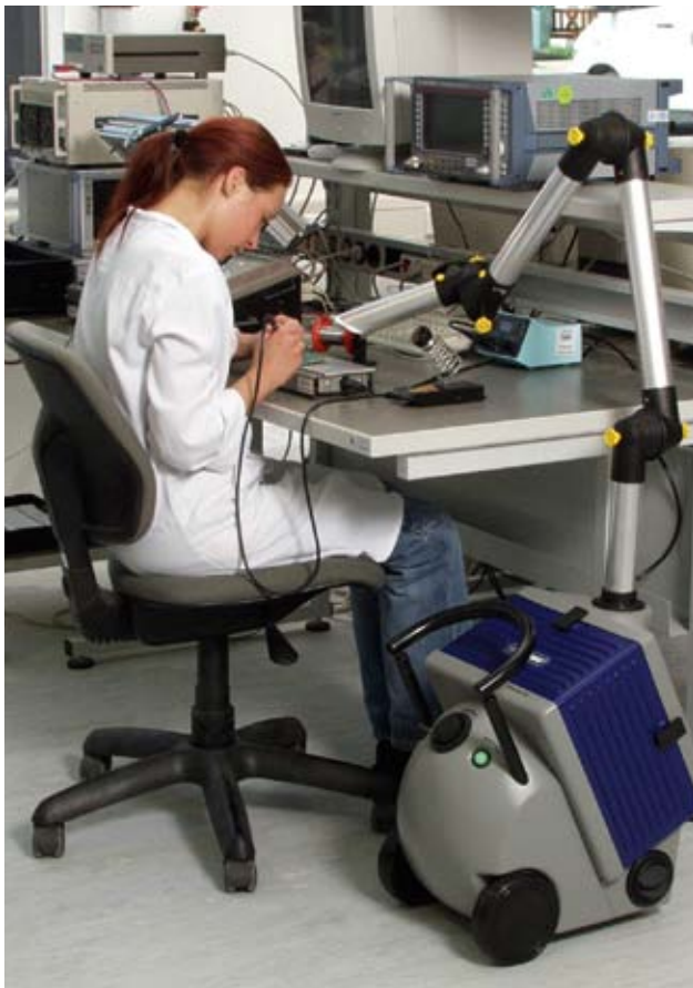
Manual soldering workstation with extraction and filtration technology.
